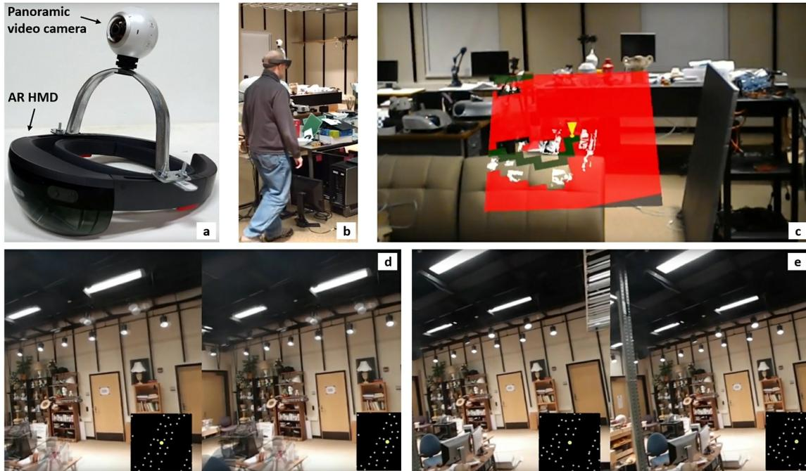
Figure 1: Acquisition device (a), AR-guided acquisition (b), acquisition map visualization (c), guided stereo VR visualization from viewpoint in between acquisition locations (d), and from acquisition location (e).
