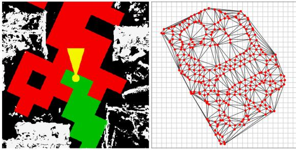
Figure 2: Left: 2D map shown to the user during acquisition. Right: 2D triangulation of panorama positions selected from acquisition path.
