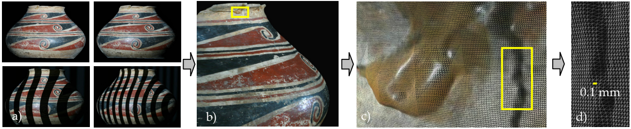
Figure 1. Photogeometric Acquisition. a) Our method captures photometric (top) and geometric (bottom) observations of an object. b) A novel viewpoint rendering of a 3D model is produced using our photogeometric method. c) A close-up of the model rendered with texture mapping. d) An even closer view of the model now rendered using wireframe and synthetic shading showing details beyond those possible using only geometric observations. Our approach uses the same hardware as standard structured-light but is fully self-calibrating and able to capture models at the resolution of the camera (in this example camera resolution is 10x greater than projector resolution). The average triangle edge length is 0.09035 or about 0.1 mm.
