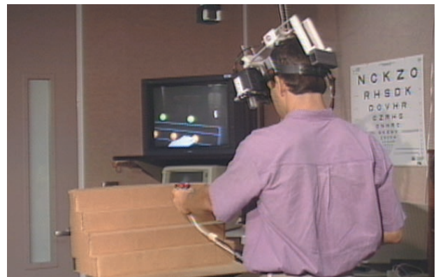
Figure 1. An augmented reality system. A see-through head-mounted display is connected to an image-generation system to present to the user a world consisting of both virtual and real objects.
