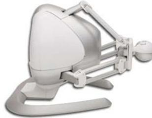
**Fig. 1.** The Falcon haptic device used in our testing.
