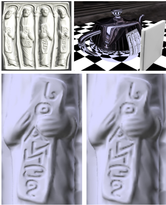
Figure 6. CoNUS depth image emphasizing all 4 engraved tablets (top left), scene setup (top right), and reflection details rendered with CoNUS (bottom left) and conv. (bottom right) depth image.
