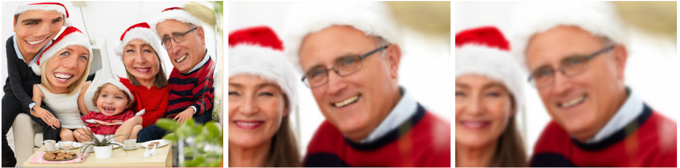
Figure 1. Coherent non-uniform sampling (CoNUS) image that allocates more samples to the face regions (left), output frame reconstructed from CoNUS image (middle), and output frame reconstructed from a conventional image (right), for comparison.
