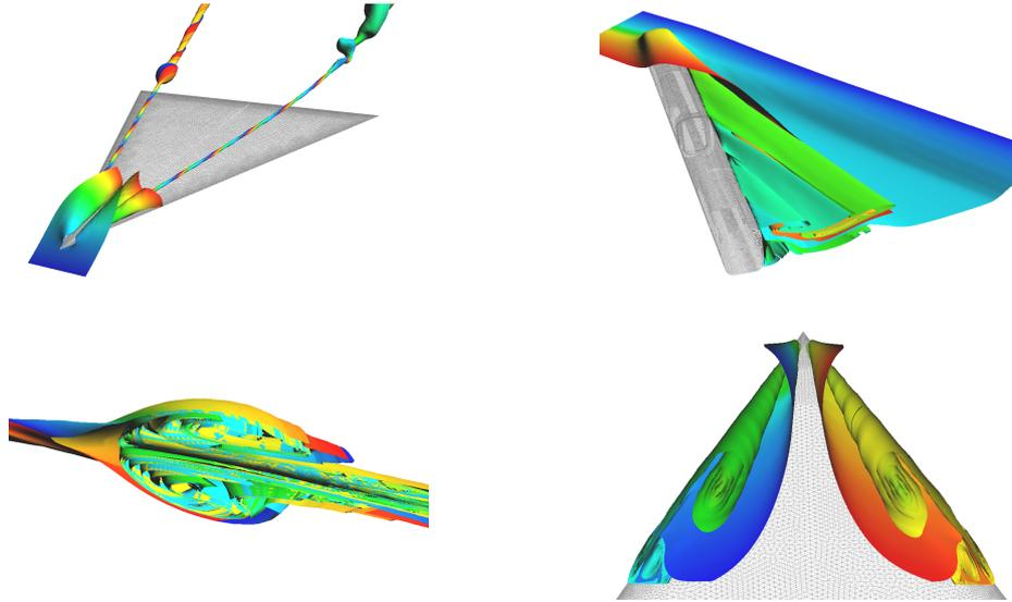
**Figure 8:** *Upper left:* Overview of the delta wing dataset with vortex creation at apex and the two primary vortices, breaking down differently. *Upper right:* Stream surface around ICE train showing vortices on the lee side. *Lower left:* Vortex breakdown cut open, revealing recirculation. *Lower right:* Formation of primary, secondary and tertiary vortices at wing apex. Note how the shape of the tertiary vortex is strongly elliptical.
