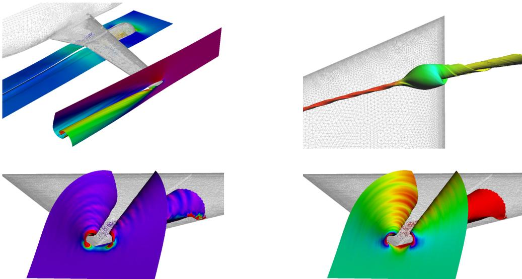
**Figure 9:** *Upper left:* Stream surfaces in the F6 dataset. Vortex generation at the wing. *Upper right:* Stream surface showing vortex breakdown, helicity magnitude color mapping. A strong correlation between helicity magnitude and the onset of vortex breakdown is evident. *Lower row:* Apex surface in the delta wing dataset, colored according to Gaussian curvature (left) and streamline stretching (right), revealing geometric properties of the stream surface.
