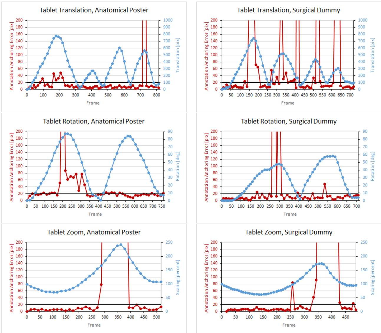
**Fig. 14** Anchoring error graphs for the tablet repositioning conditions for the sequences from Table 1. The blue lines graph the change in tablet pose, the red lines graph the error values, and the black lines show the error threshold below which tracking was considered successful.
