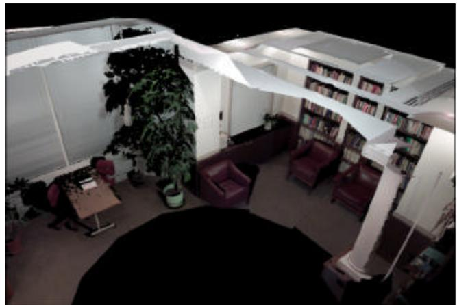
**Figure 10.** These images were rendered with the WarpEngine simulator. The reference depth images were created by registering color images with the range information acquired by our laser range finder. The range finder captured data from two positions in the center of the room. We are missing some data, on the ceiling for example.
