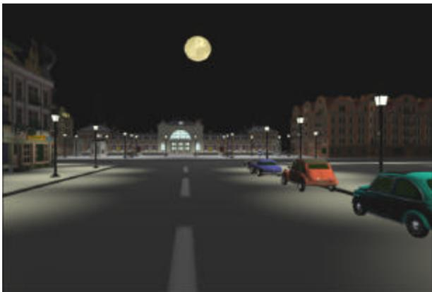
**Figure 5.** Eurotown images were made from reference depth images placed on a regular grid. Only the reference images of the current grid-cell were used to render each frame.
