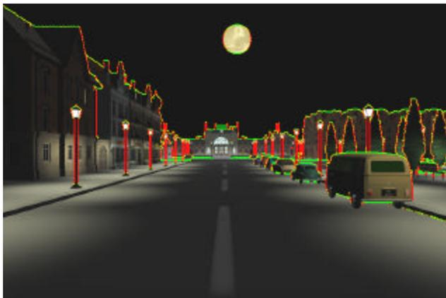
**Figure 2.** The vertical and horizontal depth discontinuities are marked in green and red, respectively. The detection algorithm works well in spite of the great range of distances in the image.
