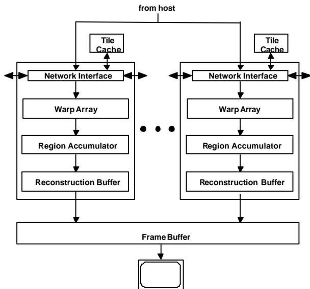
Figure 7. Block diagram of the WarpEngine
