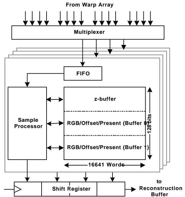
Figure 9. Block diagram of the Region Accumulator
