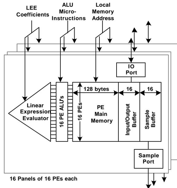
Figure 8. Block diagram of the Warp Array
