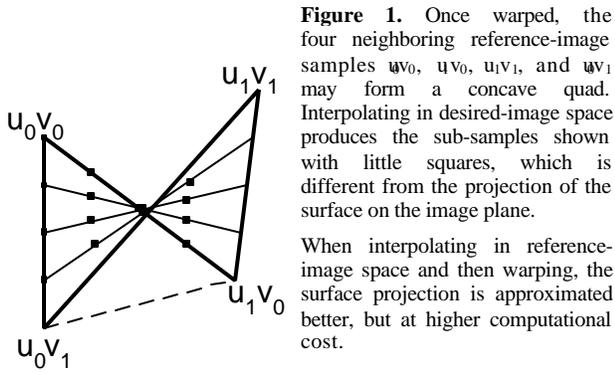
**Figure 1.** Once warped, the four neighboring reference-image samples  $u_0v_0$ ,  $u_1v_0$ ,  $u_1v_1$ , and  $u_0v_1$  may form a concave quad. Interpolating in desired-image space produces the sub-samples shown with little squares, which is different from the projection of the surface on the image plane.
