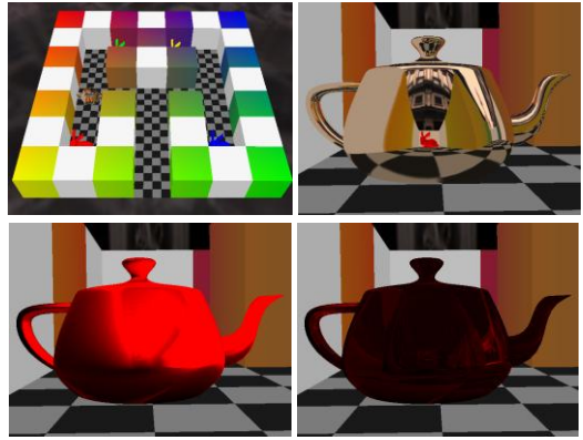
Figure 19. Teapot location and reflection (top), and number of steps visualization (bottom) w/o and w/ coarse stepping. Brighter red indicates a large number of steps being taken.
