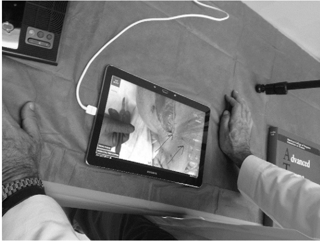
FIGURE 4. A remote surgeon provides guidance using STAR to provide telementored guidance to a local surgeon. Annotations (dark arrows) were drawn by the remote user and transmitted to the local surgeon's view of the operating field.
