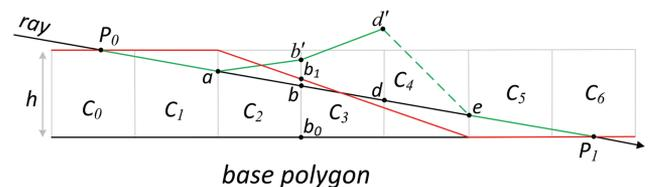
Figure 14: Intersection between ray and grid cells ( $c_0$  to  $c_6$ ). The red line shows the height of the 3-D detail tapering off over cells  $c_2$  to  $c_4$ . The green line shows the virtual ray modification that implements the tapering of 3-D detail.
