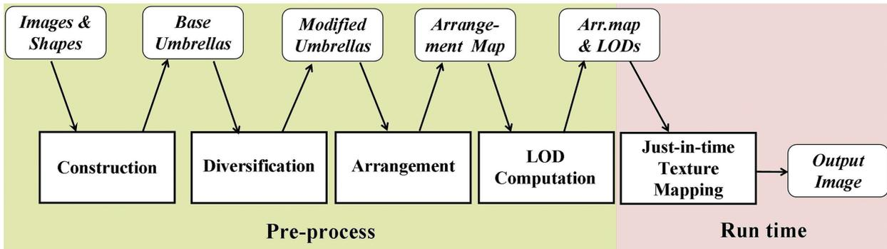
Figure 4: Overview of the just-in-time texture synthesis pipeline.
