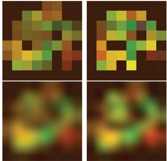
**Figure 11:** Comparison between minification with our LoD algorithm (left) and with mipmapping (right).
