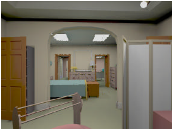
Color Figure C: Layered Depth Image. The LDI for the portal captures almost all of the visible detail. In addition, it takes up less storage and can be rendered faster than two full reference images. Furthermore, in the architectural domain, we can construct high-quality LDIs by using reference images sampled along a semicircle in front of each portal.
