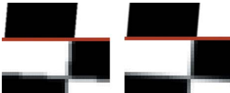
Fig. 17(b). Image obtained without (left) and (right) offsets. The 8 \times 8 magnifications in the bottom row show that offsets correctly create intermediate levels of grey which alleviate the jaggedness of the edges of the squares.
