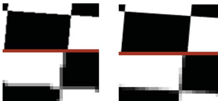
Fig. 28. Forward rasterization with one color sample per pixel, without (left) and with 4 \times 4 offsets (right). The bottom half of each image is an 8 \times 8 magnification of a fragment of the top half. Both images are reconstructed with a 2 \times 2 raised cosine kernel which for the left image is equivalent to arithmetic averaging.
