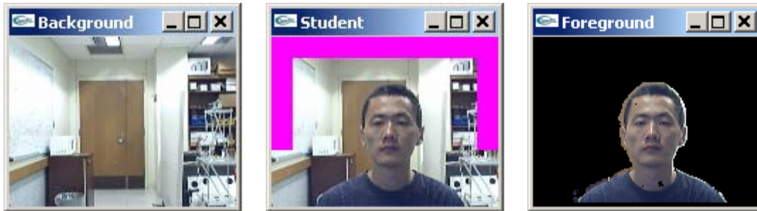
Figure 8. Frame, background, and video sprite compute by background subtraction.
