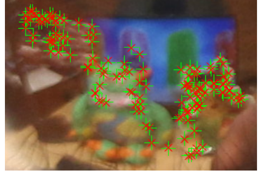
Figure 8: Detected features (green) and reprojected features (red). The average reprojection error is 0.54 pixels.
