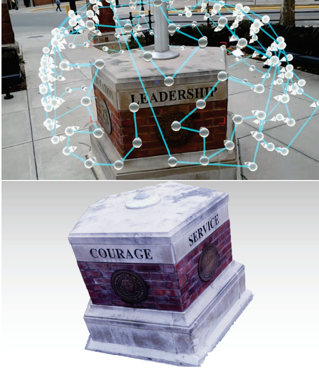
Figure 5: An example of our AR HMD guided acquisition functioning in an outdoor environment. Top: Suggested views and acquisition path. Bottom: High quality photogrammetric reconstruction.
