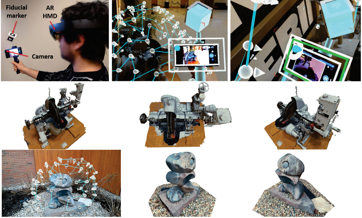
Figure 1: Top left: Our acquisition guidance system, made up of an AR HMD and a handheld camera rig tracked using a fiducial marker. Top middle: Operator AR view of scene, with virtual overlay of camera rig, automatically-generated suggested views (white icons), and suggested acquisition path (blue lines). Top right: Interactive guidance (green rectangle) for precise 6-DOF alignment of camera rig with suggested view. Second row: Photogrammetric reconstruction of scene from images captured during guided acquisition. Third row: AR view of suggested views on outdoor scene, and photogrammetric reconstruction from acquired views.
