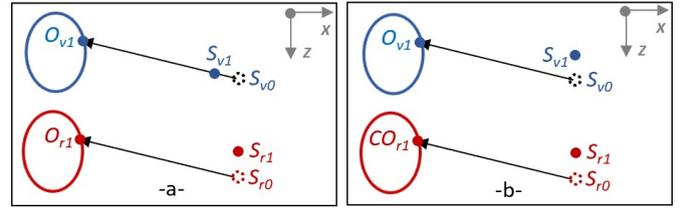
Fig. 4. Updating the virtual stick contact point  $S_v$  with a naive (a) and with our (b) algorithm. Virtual entities are shown in blue and real entities are shown in red. The naive algorithm results in a motion of the virtual stick that is different from that of the real stick. Our algorithm conveys to the user a sense that they are controlling the virtual stick, which moves in a way similar to the real stick.
