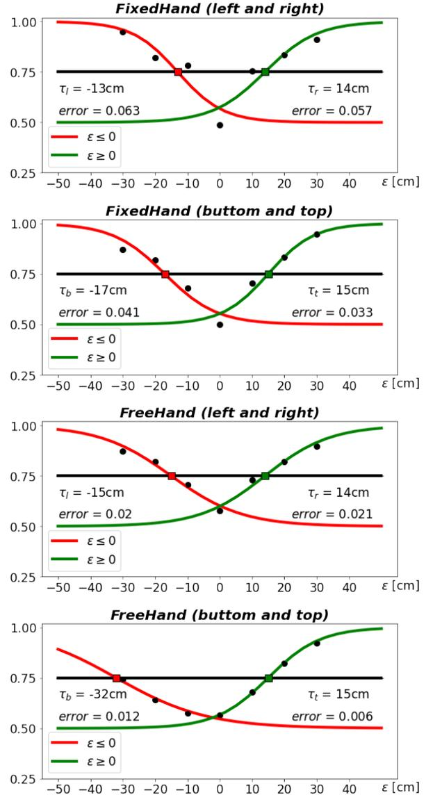
Fig. 7. Detection thresholds for the two redirection methods:  $\tau_l$  and  $\tau_r$  for left and right offsets, and  $\tau_b$  and  $\tau_t$  for bottom and top offsets. For each graph, the y axis is the percentage of correct answers and the x axis is the offset between the real and virtual objects.
