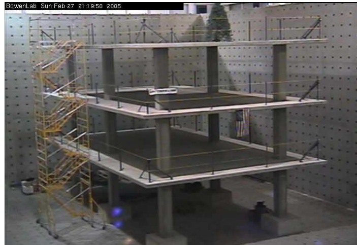
Fig. 6. Image of the test structure ( 30 \times 50 \times 35 feet) at the Bowen Lab for Structural Engineering at Purdue University. The structure will be subject to a variety of external loads and responses will be used to validate model reduction and simulation frameworks. A live web-cam image of this structure is posted at http://newton.ecn.purdue.edu/ce/Bowen/Webcam/ .
