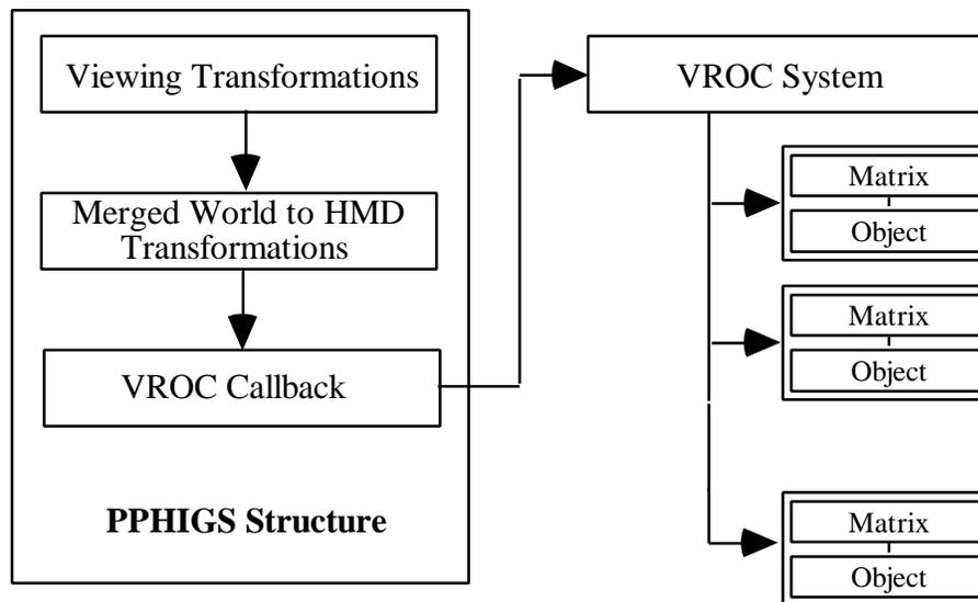
Figure 3.7: PPHIGS and VROC overall data structure
