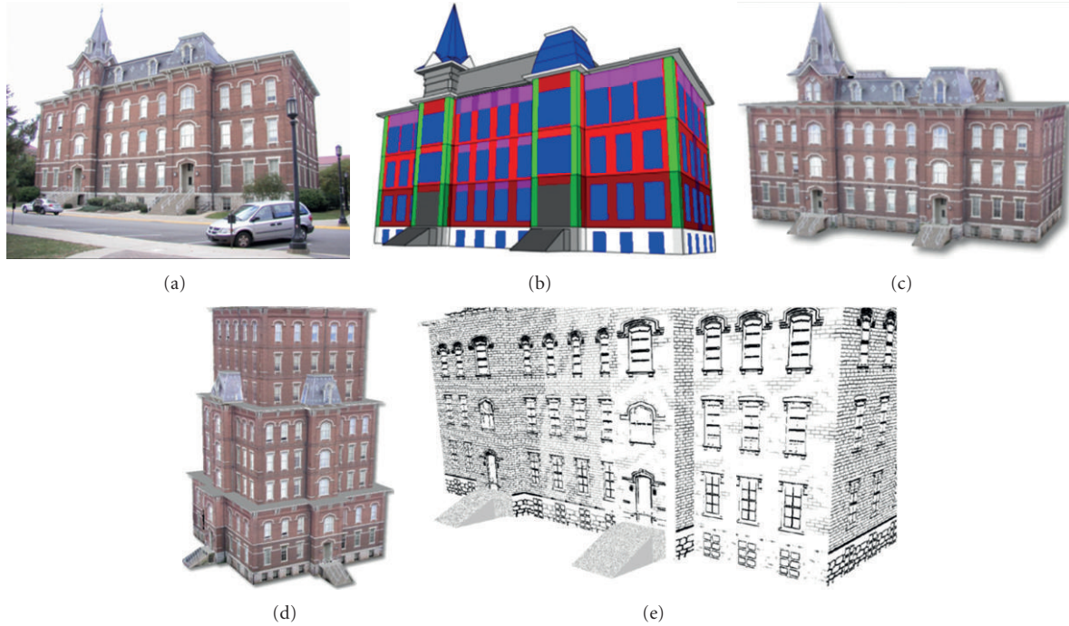
FIGURE 9: Inverse building modeling. An example of inverse building modeling of known rules but unknown parameter values. (a) One of several input photographs. (b) Manually labeled building model from which rule application and parameter values are automatically inferred. (c) Regeneration of the same initial building model. (d) Generation of a different building in the same style. (e) Nonphotorealistic rendering possible by altering only the terminal symbols of the inferred procedural model (image from [10]).
