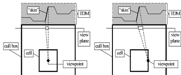
**Figure 3.** TDM Error Metric. (Left) Skin as seen from center of virtual cell. (Right) Skin as seen from the cell boundary. TDM error metric measures the maximum skin size, in screen-space pixels, for each cell.
