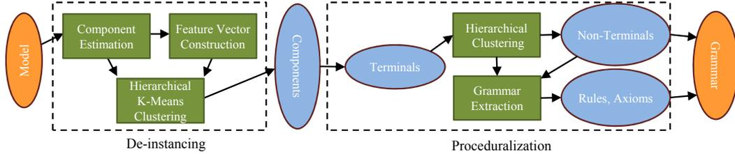
Figure 2. **Pipeline.** From the input model, we perform de-instancing to obtain component types which are then given to proceduralization (hierarchical clustering and grammar extraction) to output a grammar for the city.
