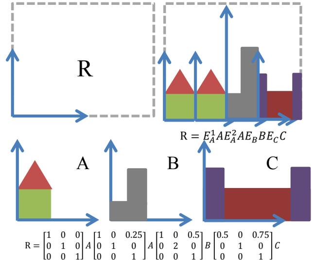
Figure 5. **Grammar Example.** A pictorial 2D example for a rule  $R \rightarrow AABC$ . The space of a non-terminal is filled with components A, B and C, using the average transformation matrices shown in Rule R.
