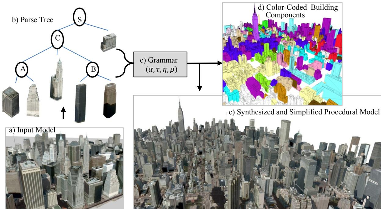
Figure 1. **City-Scale Building Proceduralization.** Our approach uses a) an unorganized 3D model as input, b) computes a hierarchical clustering of building components, and c) extracts a context-free grammar of the urban area. We can procedurally generate (d-e) structurally-similar cities, at a chosen de-instancing level
