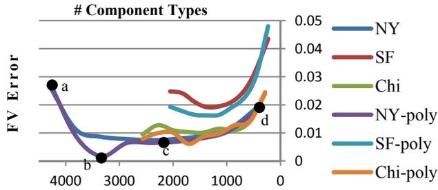
Figure 7. **Quality vs. Compression.** We show a progression of processing New York, by changing  $t_d$ . a) Original. b) De-instanced to valley of cost/benefit ratio when choosing representative component with least number of polygons. c) De-instanced with mid-range threshold and d) larger threshold. (b) and (c) have almost same visual quality yet (b) has 1/10 of the polygons of (c). In (d), the city converges to one average building (e.g., the root of the parse tree).
