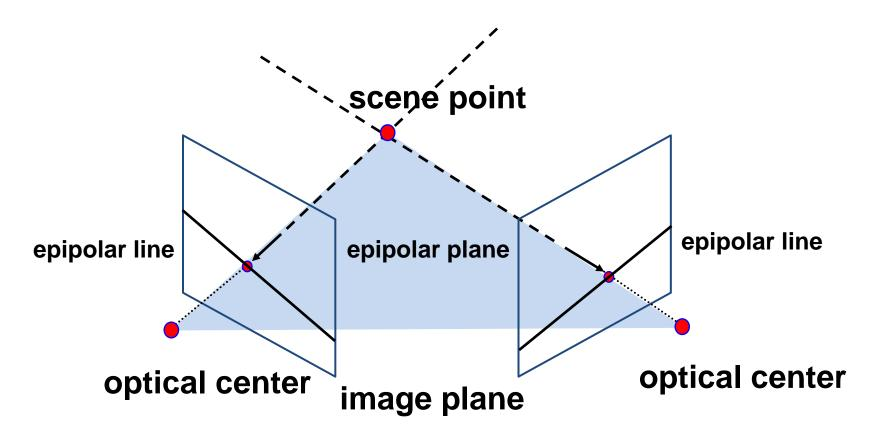
**Epipolar Constraint**: can be expressed using the fundamental matrix F
