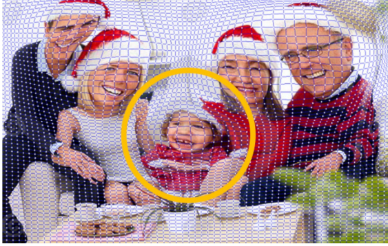
Fig. 9. Mass-spring system used to define sampling maps interactively. The user defines regions of higher resolution using a circular brush (yellow).
