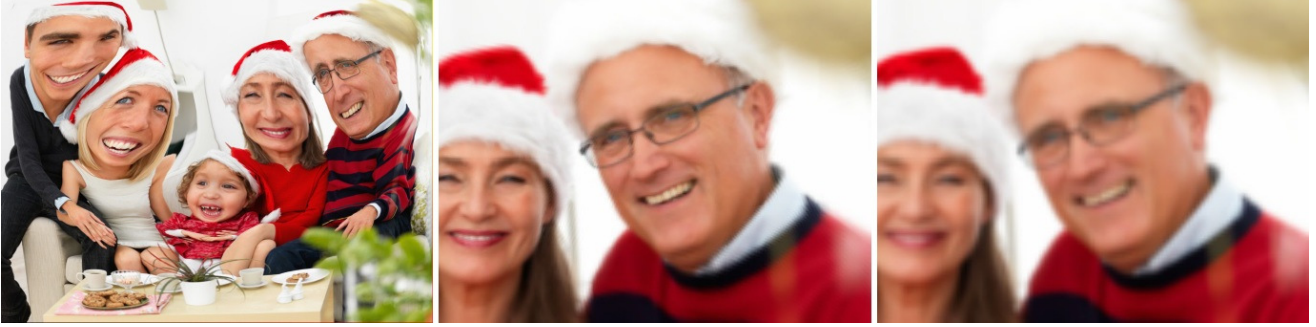
Fig. 1. Coherent non-uniform sampling (CoNUS) image that allocates more samples to the face regions (left), output frame reconstructed from CoNUS image (middle), and output frame reconstructed from a conventional image of same size (right), for comparison.
