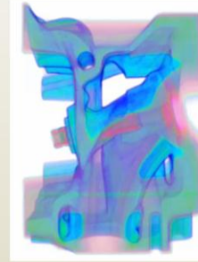
Volume rendering of block engine CT scan
