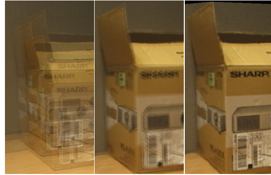
Figure 9: Images rendered from light field focused at infinity, from light field focused at the scene centroid, and from acquired model.
