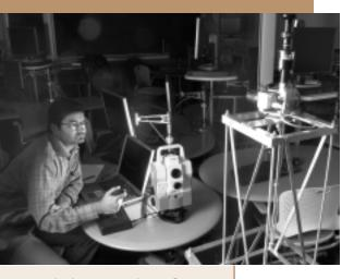
An Autonomous Image Capture pioneer robot with a laser positioning system, often used by construction engineers, collects raw images of a building and uses them to build a 3D colored model.
