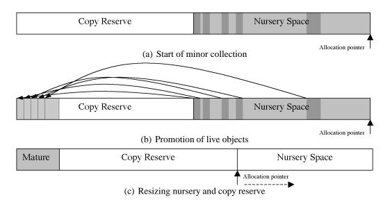
Figure 2.4. Minor collection in an Appel-style collector
