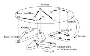
Fig. 1. Overlay internetworking architecture: An overlay internetwork is constructed among exported hosts. Long-lived fbws (dash-dot lines) in home overlays are replaced by Synergy routes (thick lines) if this will improve performance.
