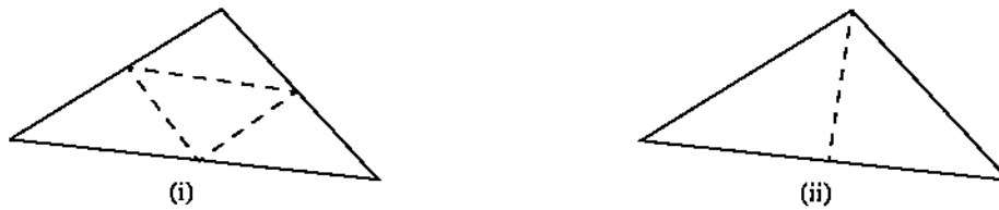
Fig. 4. Element-wise refinement of a triangle by (i) regular division and (ii) bisection.
