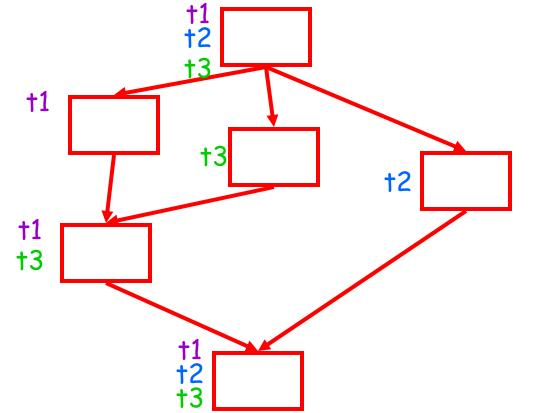
Label each node of the control flow graph with the set of tests that reach it.
