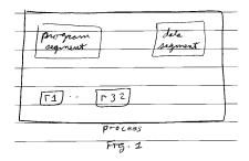
In Figure 1 the "program segment" represents the instructions to run, the "data segment" contains the heap and stack (as is depicted in Figure 2), and r1, ..., r32 are the register values.
