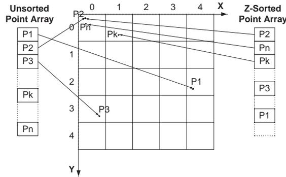
Figure 5: Example of sorted and un-sorted Object Arrays
