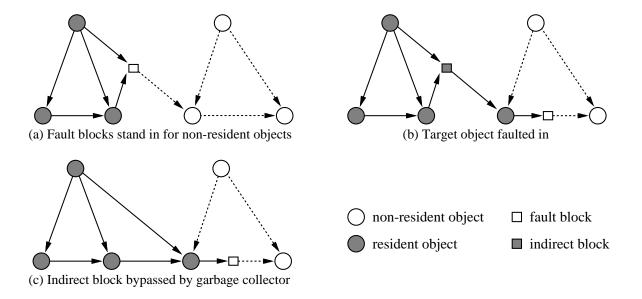
Figure 1: Fault Blocks
