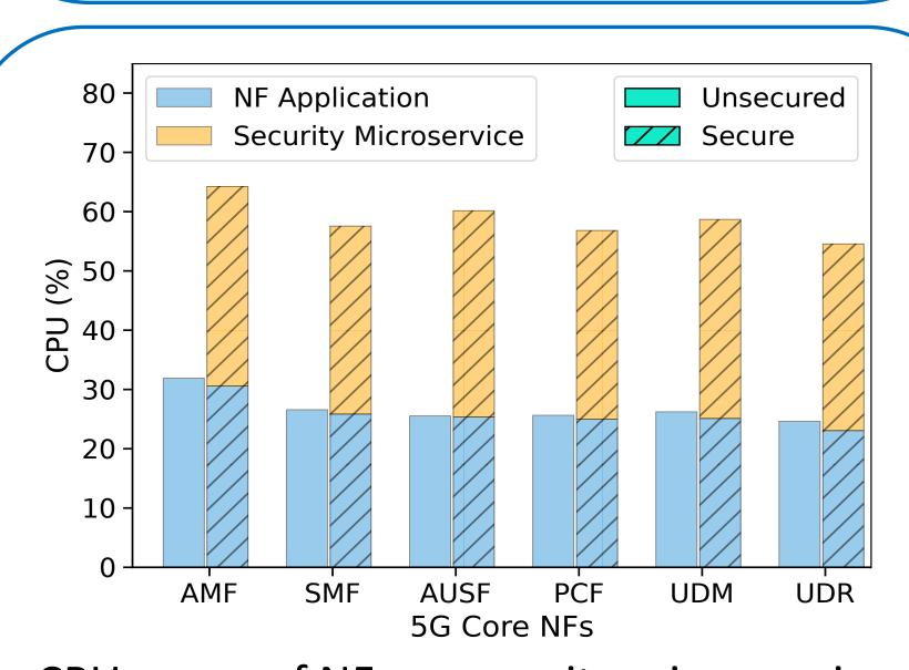
CPU usage of NF vs. security microservices
