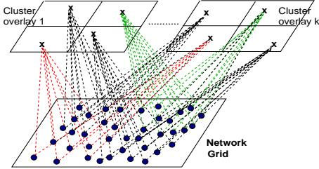
Fig. 2. A network with  $k$  cluster head overlays. Every node has one cluster head in each overlay.
