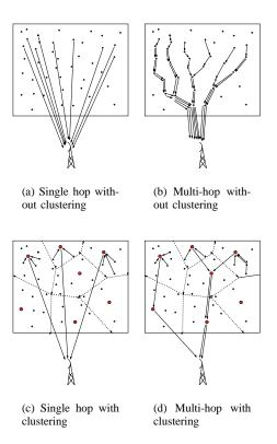
Fig. 1. Forwarding with and without clustering and aggregation
