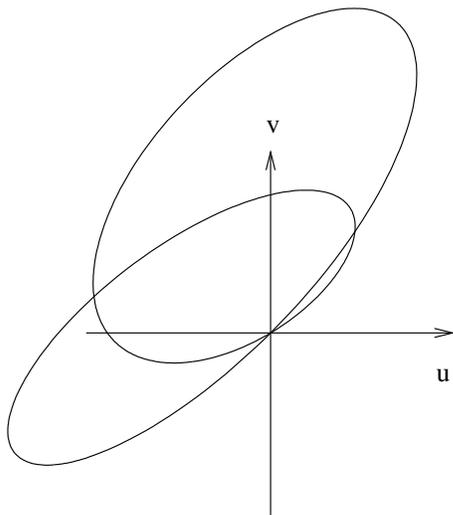
**Figure 6.12** Projection of the Cylinder/Sphere Intersection
