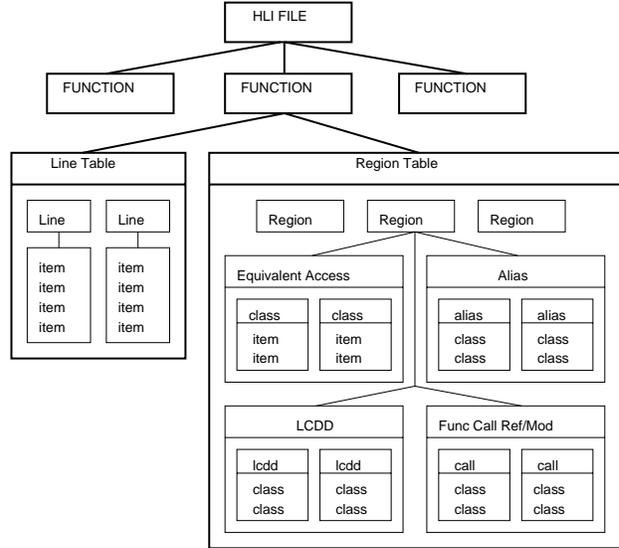
Figure 1. Top-level layout of an HLI file.
