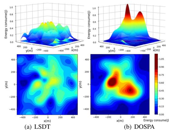
Fig. 6. Energy loss distribution diagram of nodes under the same data transmission volume.
