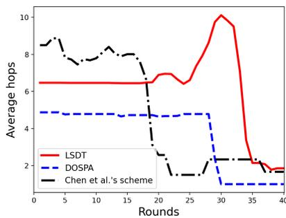
Fig. 5. The average number of routing hops during data transmission.
