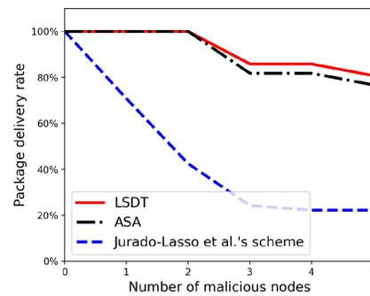
Fig. 10. The effect of resisting malicious node attacks with different number of malicious nodes.
