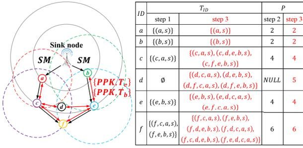
Fig. 3. The process of constructing HWSNs routing.
