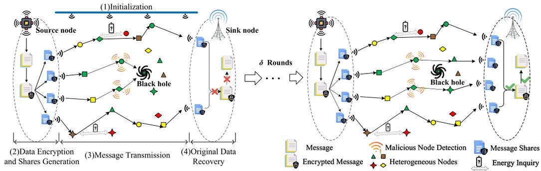
Fig. 2. Process flow of LSDT. (Take (3,4) secret sharing scheme as an example. In the left subfigure, only two routes successfully reached the sink node due to the black hole attack carried out by the malicious node, and the first round of data transmission failed. After  $\delta$  rounds data transmission, as shown in the right subfigure, the network can evade the malicious node and successfully recover the message).
