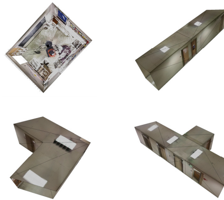
Figure 4: Four section types are fitted to the DEP data. Room section is shown with the point cloud in the top left corner.
