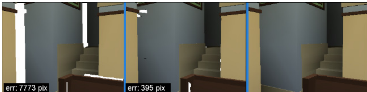
Figure 9. Three-way comparison between frames rendered from depth image, from a DDOC reference image, and from geometry.
