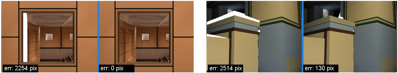
Figure 2 Pairs of frames rendered from a depth image and a DDOC reference image. Disocclusion errors are highlighted in white.
