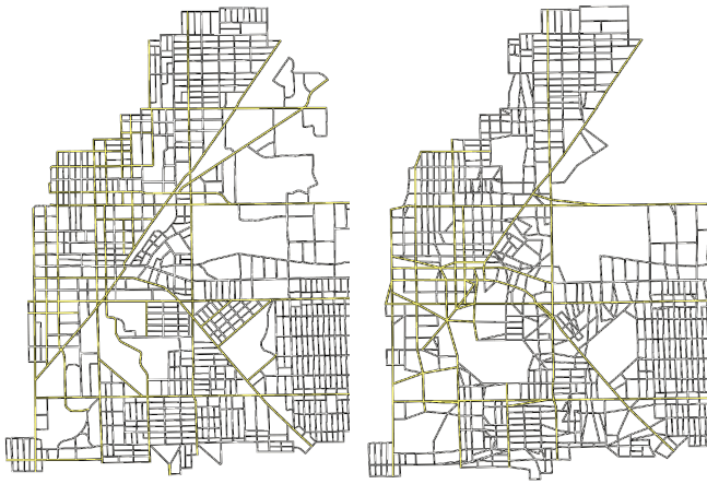
Figure 8. Abstraction into Attributed Points. The attributed intersection points of the street network of an example urban layout fragment (left) have been copied and dropped in an empty area (right). Our system is then used to connect intersection points. Notice the similarity between the reconstructed street network and the original one.
