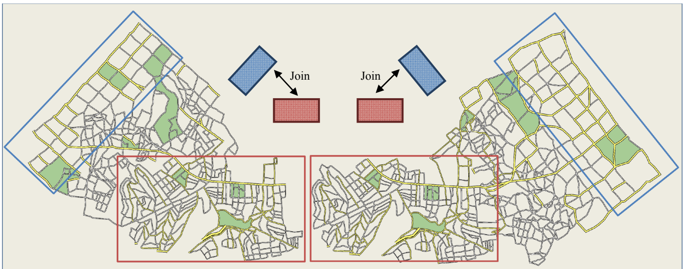
Figure 11. Join and Blend. Sequences of join and blend operations have been used to generate both street networks. In this case, the blue fragment (with grid pattern) and the red fragment (with irregular pattern) are connected in two different positions relative to each other.
