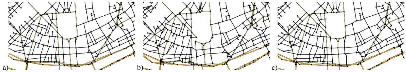
Figure 11: Effect of the grid resolution for vertex expansion on the decoded graph. The original model a) was encoded into three levels of hierarchy using grid resolution 10 \times 12 cells and decoded back b). If higher resolution of 20 \times 24 is used, the result provides better resemblance to the original c).
