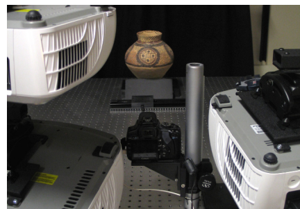
Figure 2. Object Stage. The stage used by our approach consists only of self-calibrated off-the-shelf hardware.
