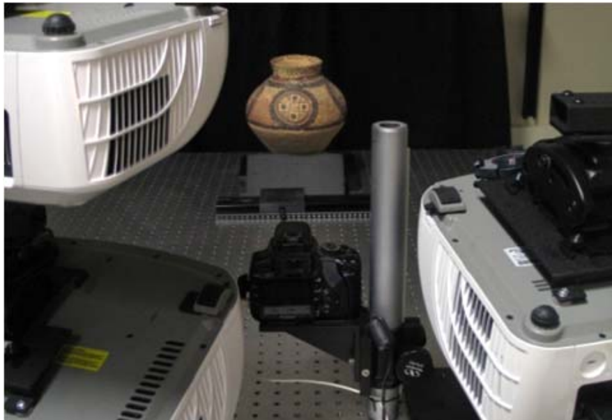
Fig. 1: Our virtual restoration system consists of self-calibrating, off-the-shelf hardware.
