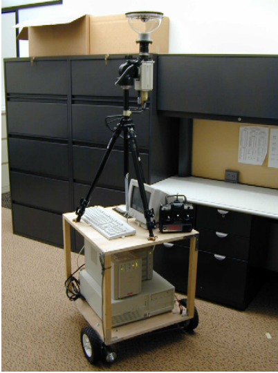
Figure 1. Camera Setup. The paraboloidal mirror is attached to the base of an acrylic dome. The dome is fastened to the video camera. The entire camera is on a radio-controlled motorized cart.
