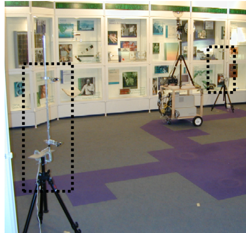
Figure 5. Example Pose Estimation Setup. The cart is placed inside an example environment for calibration and testing. The posts, outlined by boxes in the figure, are placed in the corners of the trackable region.
