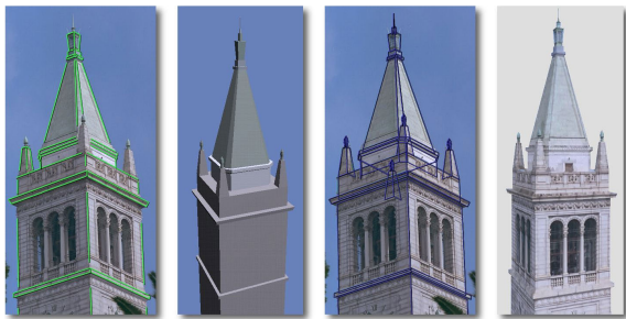
Figure 7: Interactive image-based modeling: (1) input image with user-drawn edges shown in green, (2) shaded 3D solid model, (3) geometric primitives overlaid onto the input image, (4) final view-dependent, texture-mapped 3D model. Figure courtesy of Paul Debevec [DTM96] ©1996 ACM.
