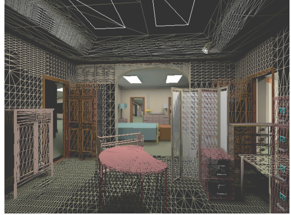
Figure 1-8. Portal-Image Culling. The portals (doorways, windows, etc.) of the current room are replaced with images, optionally warped to the current viewpoint. Consequently, the system never needs to render more than one room's worth of geometry, even if a long sequence of rooms is visible. The right snapshot shows the portal image and geometry rendered in wireframe.
