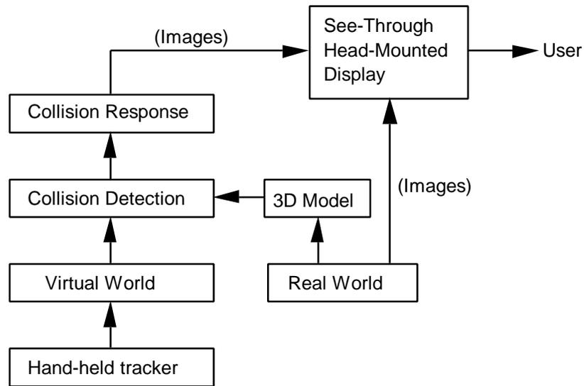
Figure 2: Schematic of entire VROC System. The user employs a 3D mouse (or hand-held tracker) to control the initial position and velocities of the virtual world objects. Collision detection and collision response is performed in the merged virtual and real world environment. Virtual imagery is combined with real world imagery in the see-through head-mounted display and presented to the user.
