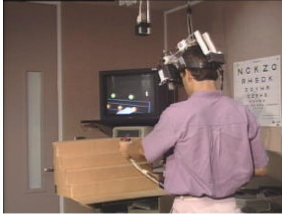
Figure 1: An Augmented Reality System. A see-through head-mounted display is connected to an image generation system to present to the user a world consisting of both virtual and real objects.
